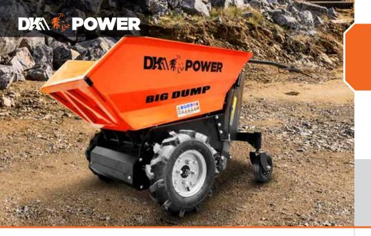
With a wet bucket for sand, gravel, concrete and more, the DK2 POWER OPD811 self-drive electric powered hydraulic dump cart runs for up to 6 hours on one charge with its 48V 20Ah battery and moves it all. Equipped with a hydraulic electric lift, this unit is capable of tipping its wet bucket 90 degrees vertically for easy unloading.
