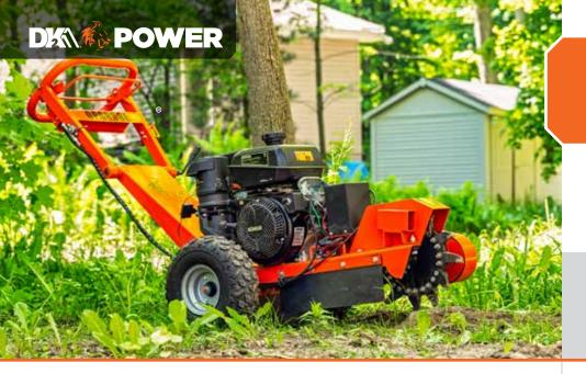
Introducing the OPG888E, powered by a KOHLER® Command PRO® CH440 14HP 429cc engine with electric start, and is capable of demolishing stumps 14 inches above ground and 10 inches below ground with its dual V-belt
