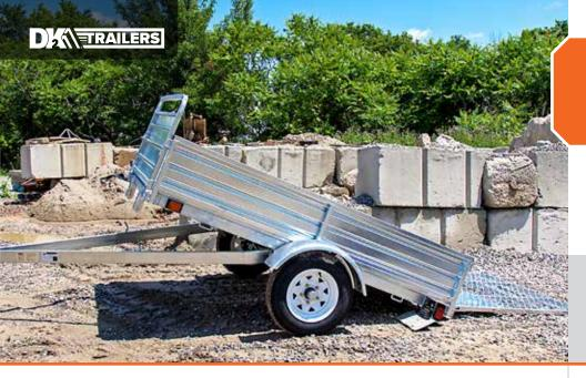
This multi-utility trailer from DK2 is one of the most versatile trailers on the market. Sitting on a solid cambered axle with 12-inch tires and a load capacity of 1,639 pounds. Equipped with a 24-inch front load-bearing gate, 40-inch rear drive-up gate, and a tilt/dump capability that makes it easy to load or unload. Fabricated from 100% hot-dipped galvanized steel, all of the components are reinforced, adjustable, removable and/or interchangeable.
