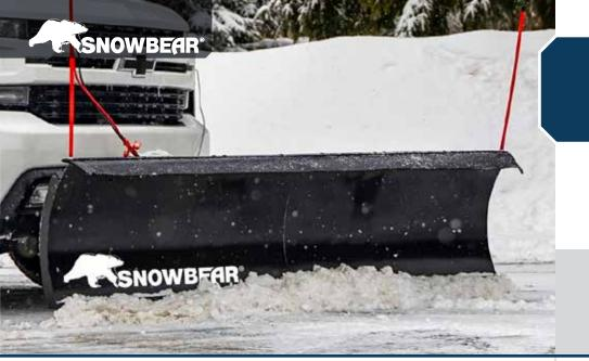
This prosumer, fully hydraulic snow plow kit provides you the opportunity to clear your parking lot, driveway, or lane way whenever required. With our fully hydraulic system you can raise, lower, and angle the snow plow blade from inside your vehicle using our wired hand held remote. For extreme durability against the elements and rust, SnowBear<sup>®</sup> combines an industrial pow-
