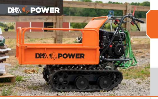
The OPD813 660 lb Gas-Powered Dump Cart with Tracks is a tool that is designed to make heavy lifting and transport easier. Powered by a KOHLER<sup>®</sup> Command PRO<sup>®</sup> CH270 7 HP 208 cc engine, with 3 forward gears and 1 reverse gear, this gas-powered dump cart can hold up to 660 pounds and has a gas rod tipping capability to make unloading quick and easy.
